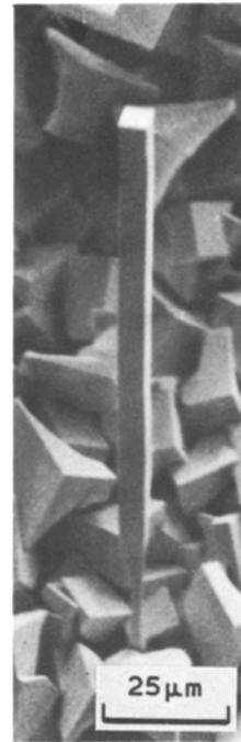
Figure 3 Connection of the whiskers with the layer.
