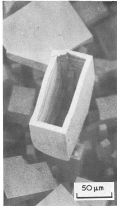
Figure 5 Hollow crystal with closed surrounding surface.
