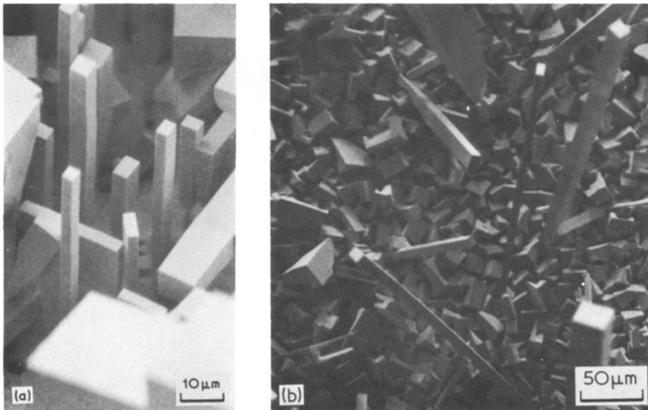
Figure 2 PbSe whiskers grown on the surface of an epitaxial layer.
