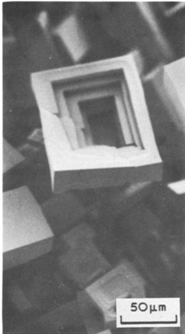
Figure 4 Skeletal crystal consisting of a whisker and a hollow four-walled pyramid.
